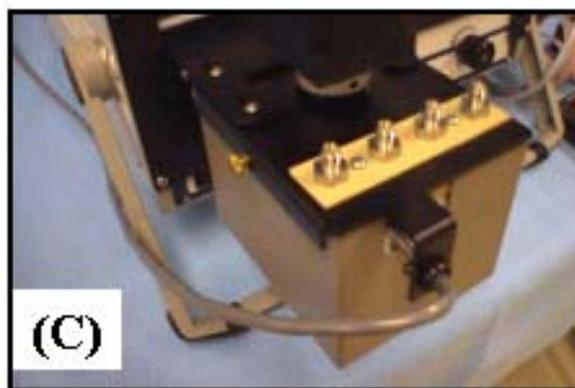
**Figure 4.** The zNose® ultra-fast GC design (A) re-configured as fully automatic chemical process controller (B & C) with a selectable multi-port inlet for measuring and controlling up to 16 multiple vapor sources.
