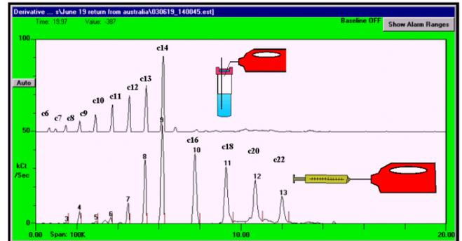
**Figure 5.** Typical n-alkane chromatogram response of a GC/SAW system
