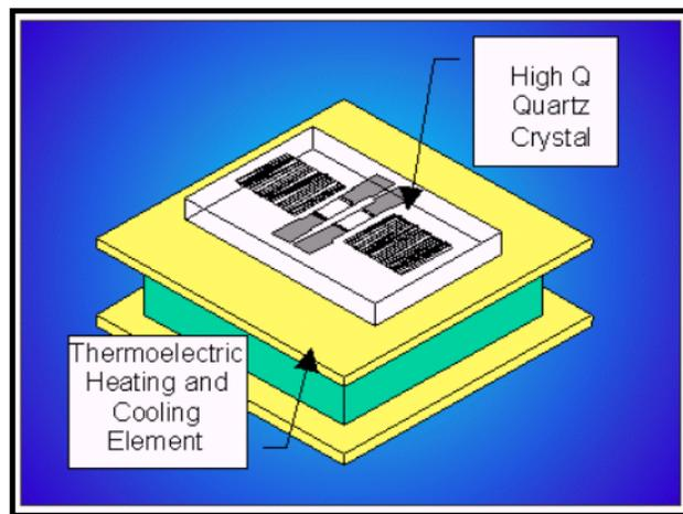
**Figure 2.** Design details of surface acoustic wave (SAW) detector.
