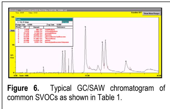
**Figure 6.** Typical GC/SAW chromatogram of common SVOCs as shown in Table 1.
