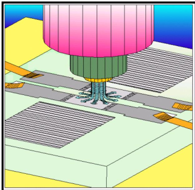
**Figure 3.** Surface acoustic wave GC sensor with nozzle details.
